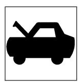
Pull the interior hood release handle with this symbol on it. It is located to the left of the parking brake pedal.
